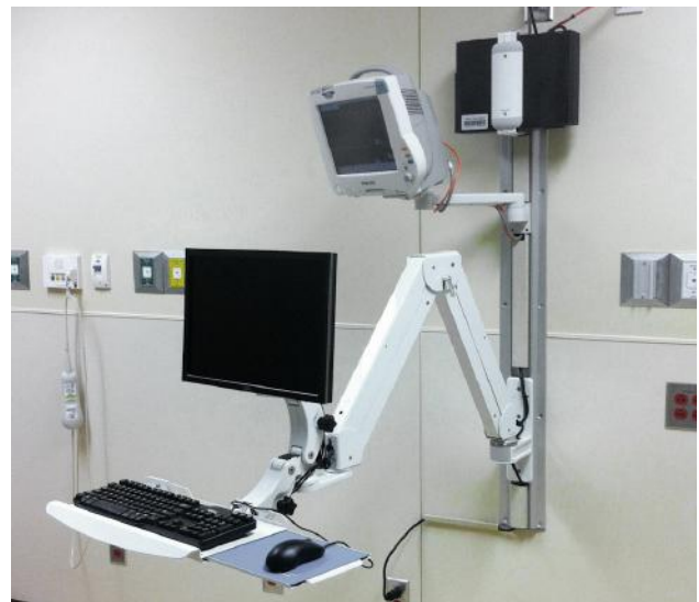
Placement of medical device on ICW track
